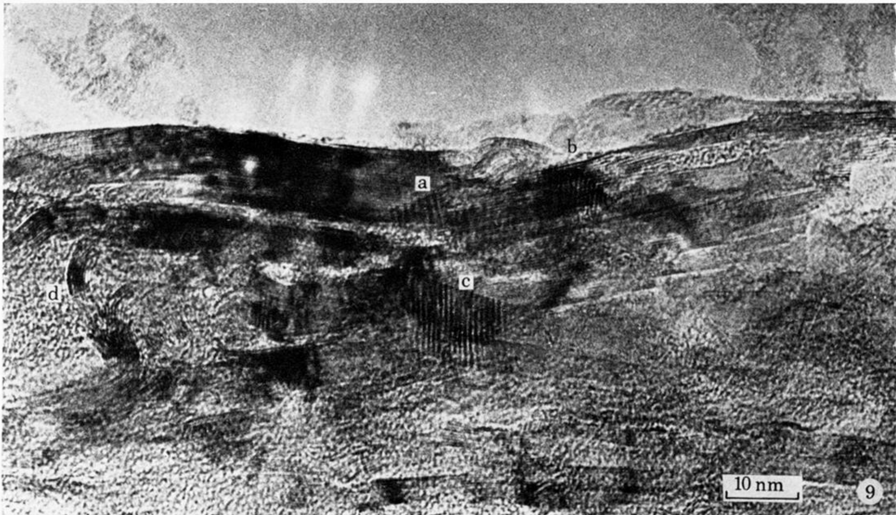
FIGURE 9. Lattice-fringe image from longitudinal section of PAN-based type I (2500 °C) carbon fibre, showing surface layers and misoriented crystallites in the skin.
